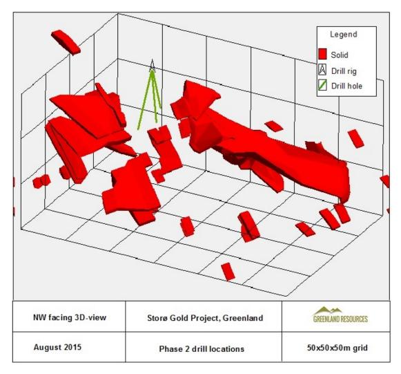
**FIGURE 1.** 3D-view of the Storo solids in red with some proposed Phase II drill hole locations in green.
